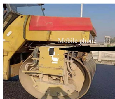
Fig. 2. Mobile phone attached to the vibratory roller drum.
