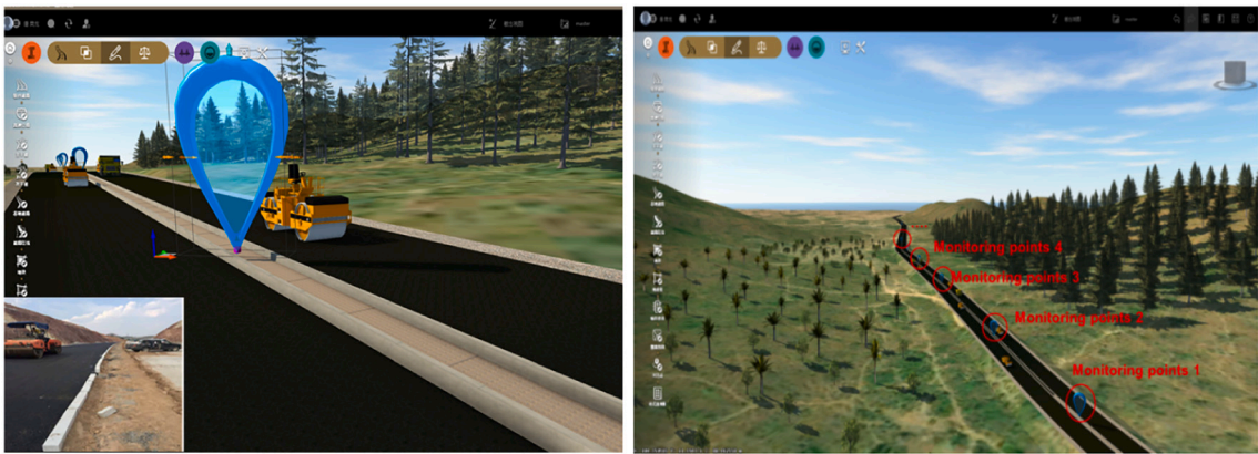
Fig. 15. Local quality monitoring by Infracore (BIM).
