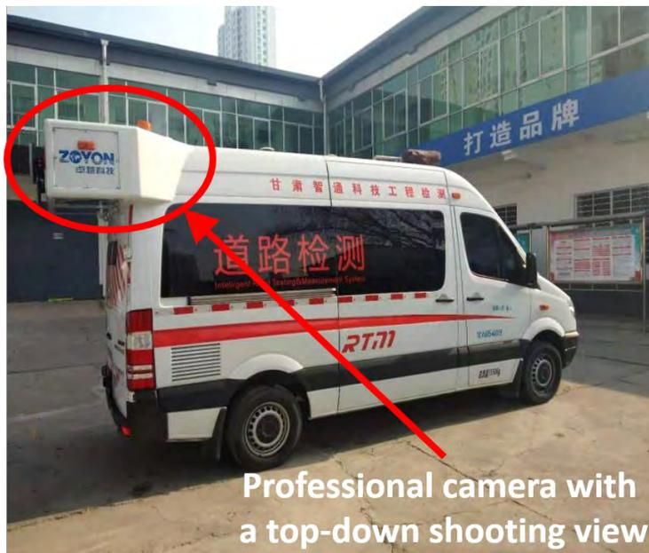
Figure 4: Multi-function detection vehicle equipped with a professional camera.
